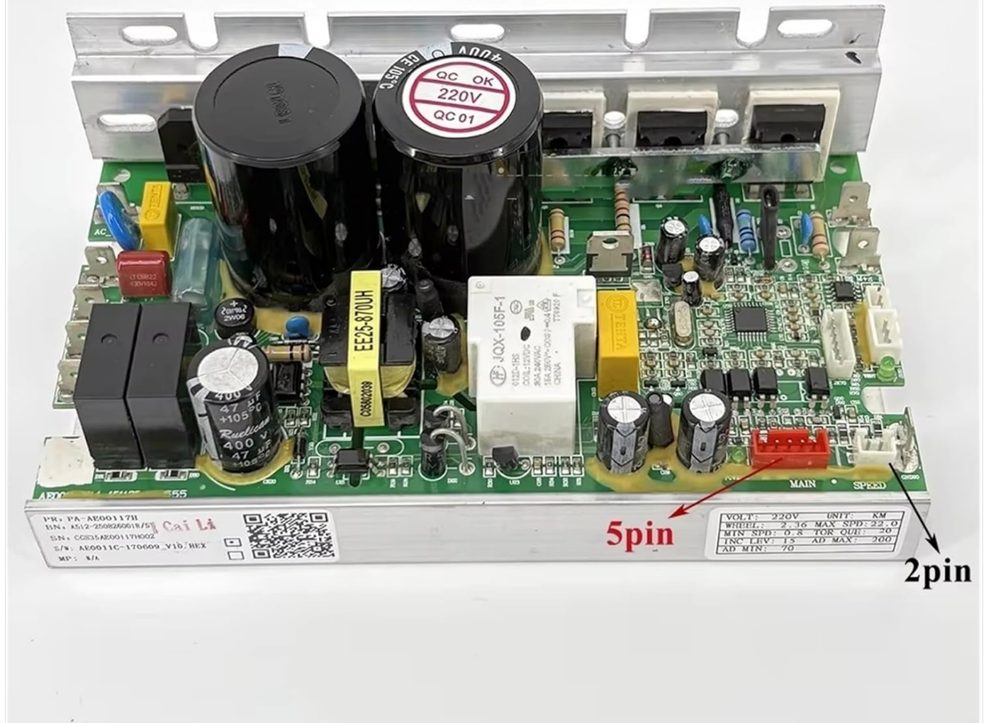
Figure 3.1: Top-down view of the AE0011C PA-AE0017H Treadmill Motor Controller. This image highlights the main components and the overall layout of the circuit board, including the large capacitors and various connectors labeled "5pin" and "2pin" for motor and sensor connections.
