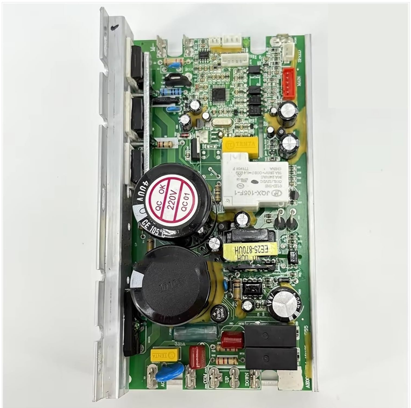
Figure 3.2: Angled view of the motor controller, showcasing the heat sink on the side and the arrangement of components from a different perspective.
