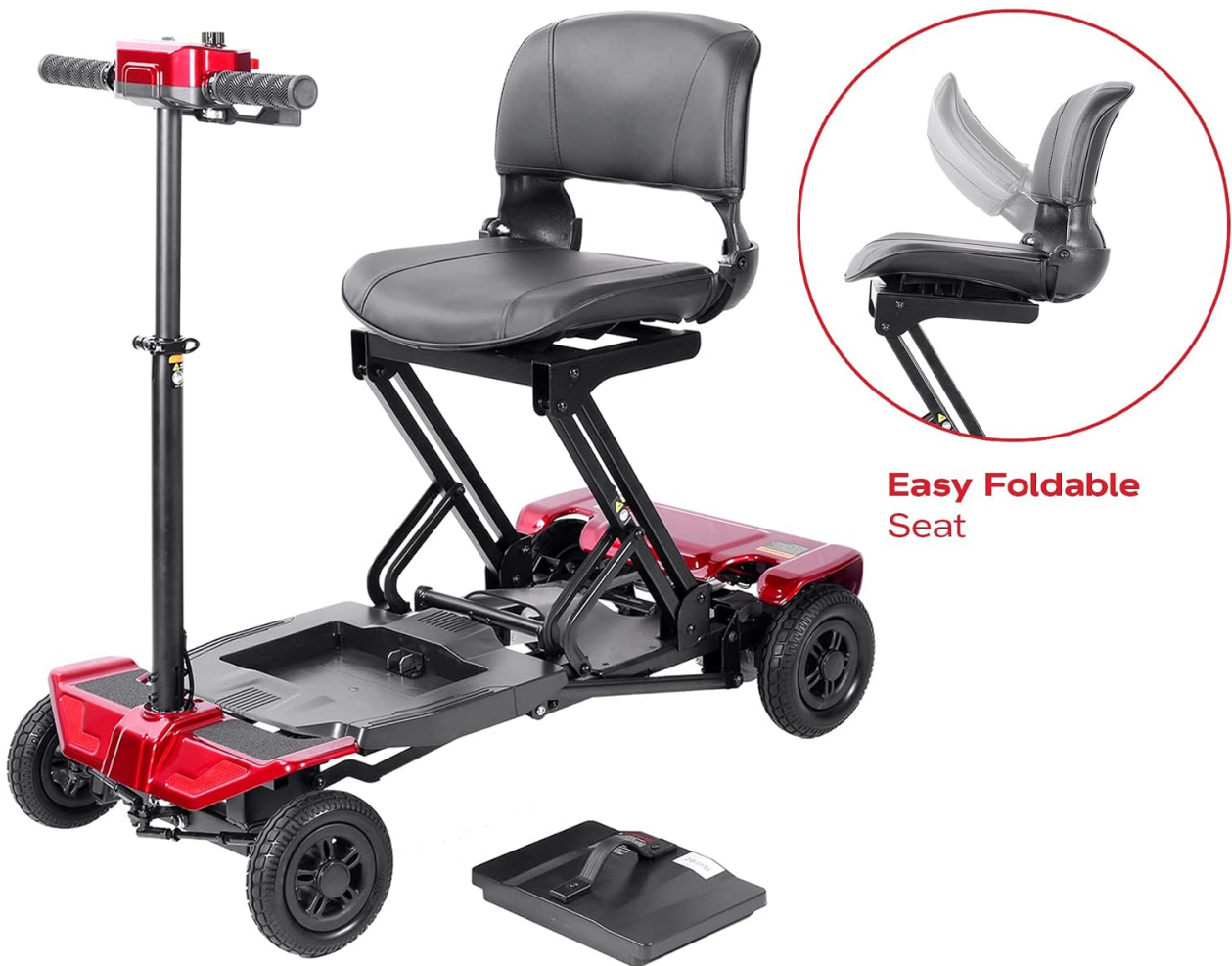
Figure 4.2: Detachable battery and foldable seat for convenient setup and storage.
