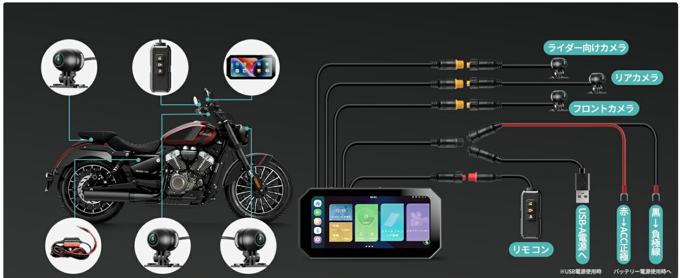
Figure 3.4: Diagram illustrating the power connection points for the drive recorder.
