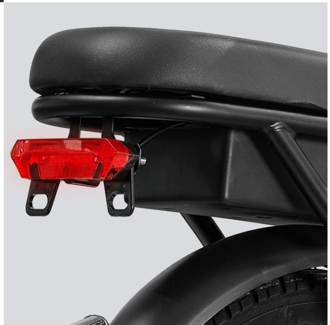
Figure 3.7: The integrated headlight and rear warning lights, designed to provide illumination and increase rider visibility for safety during day and night.
