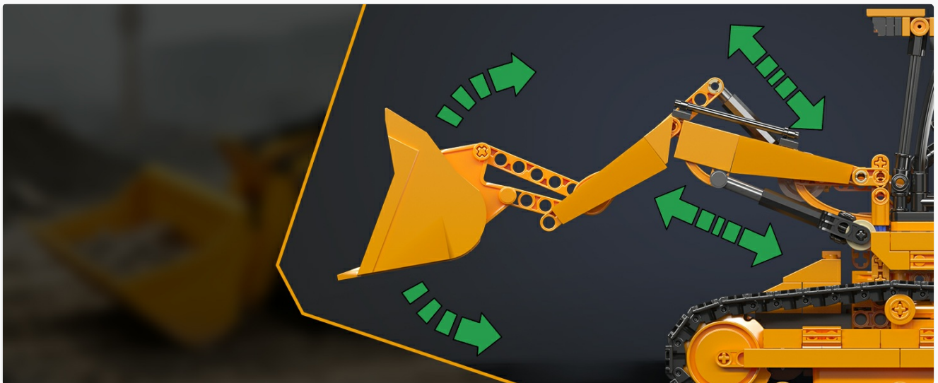
Figure 3.2: Depiction of the front blade's operational movements.
