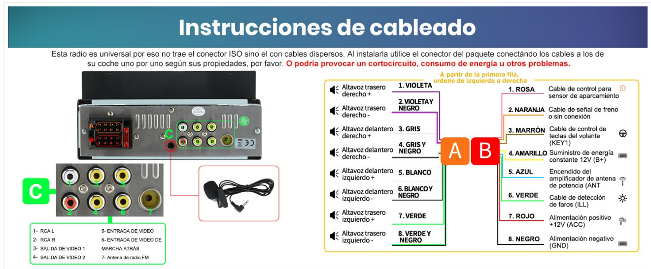
Figure 4.2: Main Wiring Diagram.
