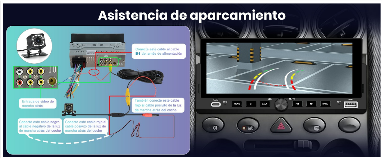
Figure 4.3: Rear Camera Wiring for Parking Assistance.
