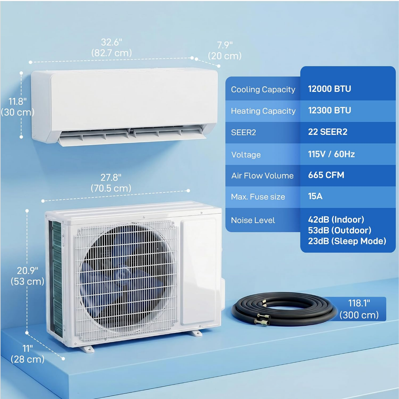
Image: Detailed specifications including dimensions of indoor (82.7W x 30H x 20D cm) and outdoor (70.5W x 53H x 28D cm) units, cooling capacity (12000 BTU), heating capacity (12300 BTU), SEER2 (22), voltage (115V/60Hz), airflow volume (665 CFM), max fuse size (15A), and noise levels (Indoor 42dB, Outdoor 53dB, Sleep Mode 23dB).
