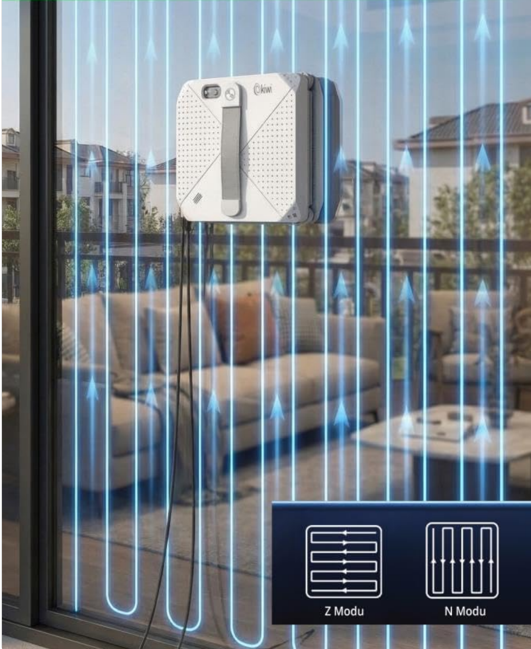
Figure 4.2: The robot utilizes intelligent scanning with Z-mode and N-mode patterns for comprehensive cleaning coverage.
