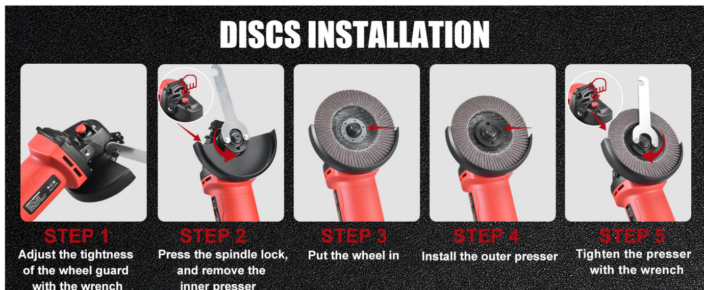
Figure 3: Disc installation steps.
