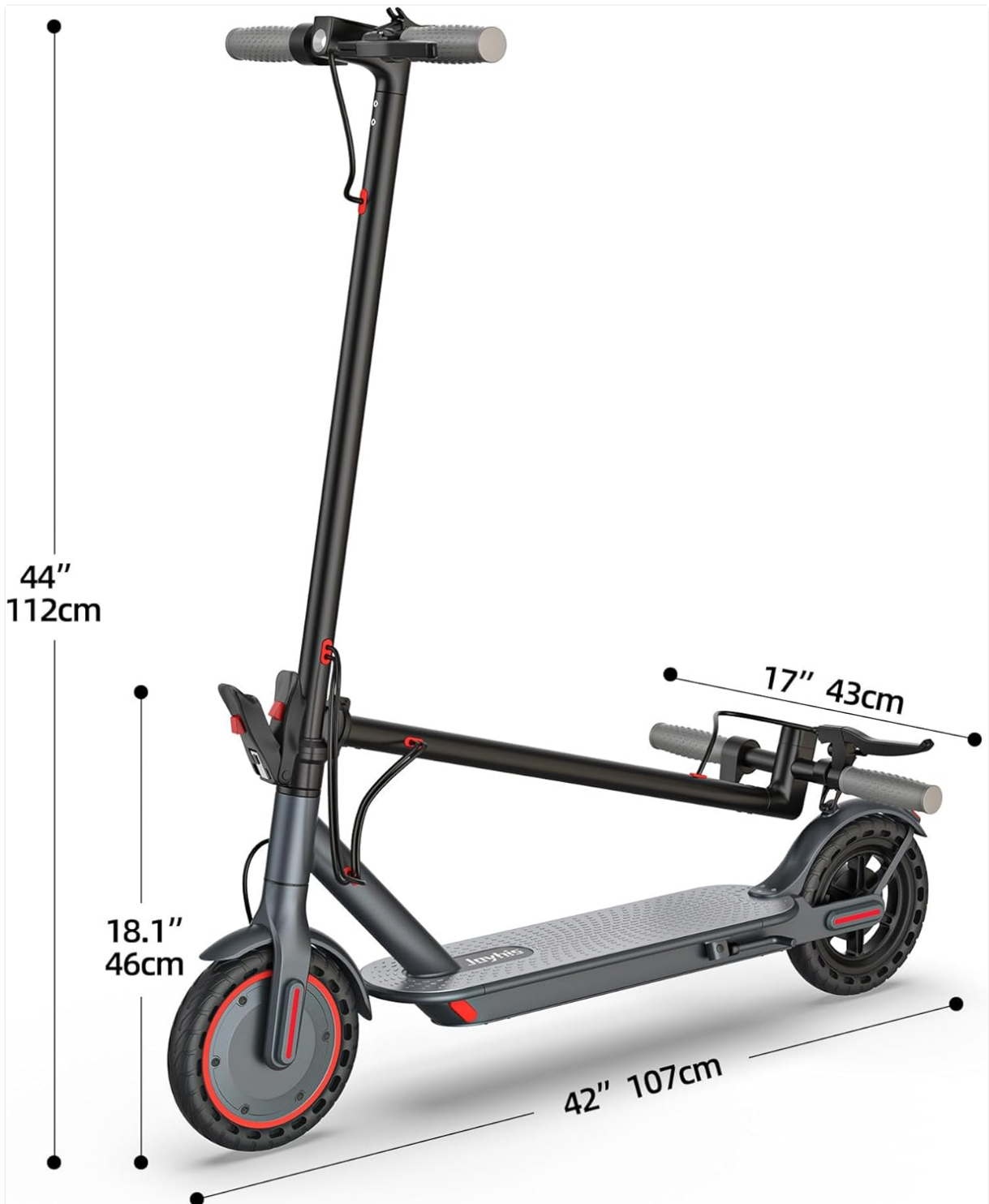
Figure 5.1: Maintenance-free honeycomb solid tire.
