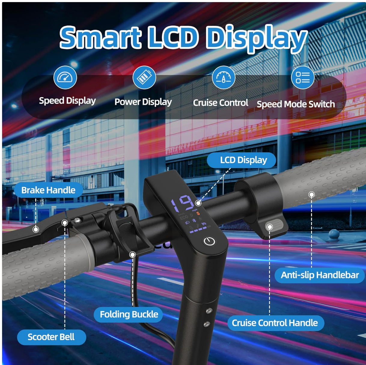
Figure 4.1: Smart LCD Display and handlebar controls.
