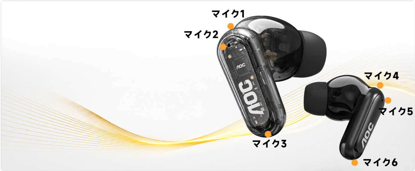
Image: Detailed view of an earbud showing microphone placement.
