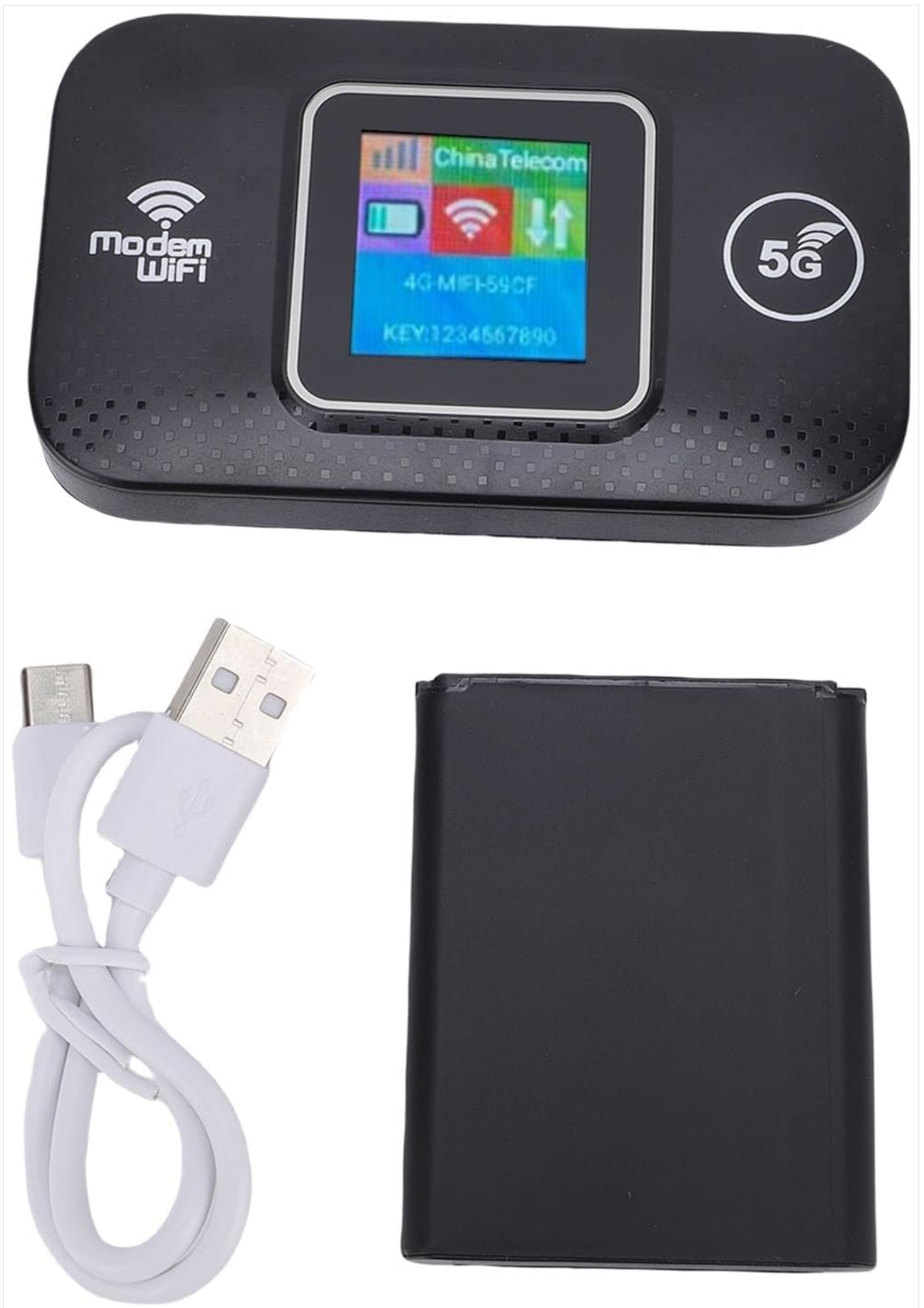
Image: The Jectse 5G LTE Mobile Hotspot Router, its USB charging cable, and the removable battery, illustrating the main components included in the package.
