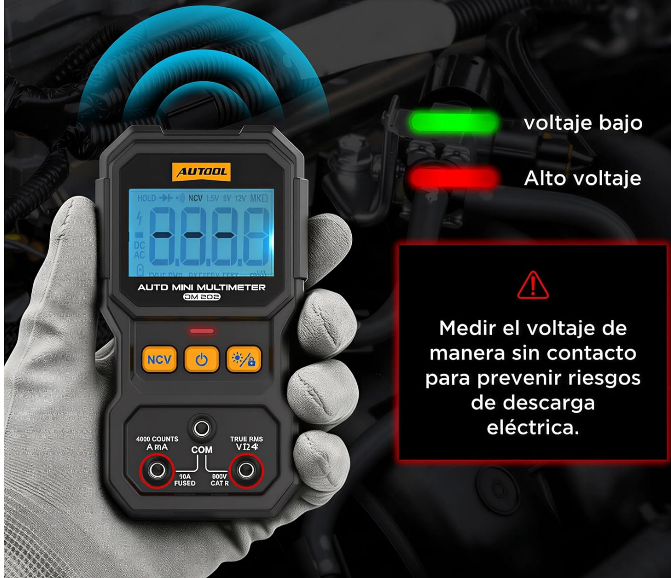
Figure 5.2: Non-Contact Voltage (NCV) detection in action.
