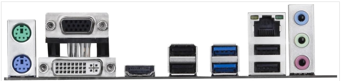
Figure 2: Rear I/O panel of the Generic B85 M-ATX Motherboard. Ports include PS/2 for keyboard/mouse, VGA, DVI, HDMI, USB 2.0, USB 3.0, RJ45 LAN, and audio jacks.
