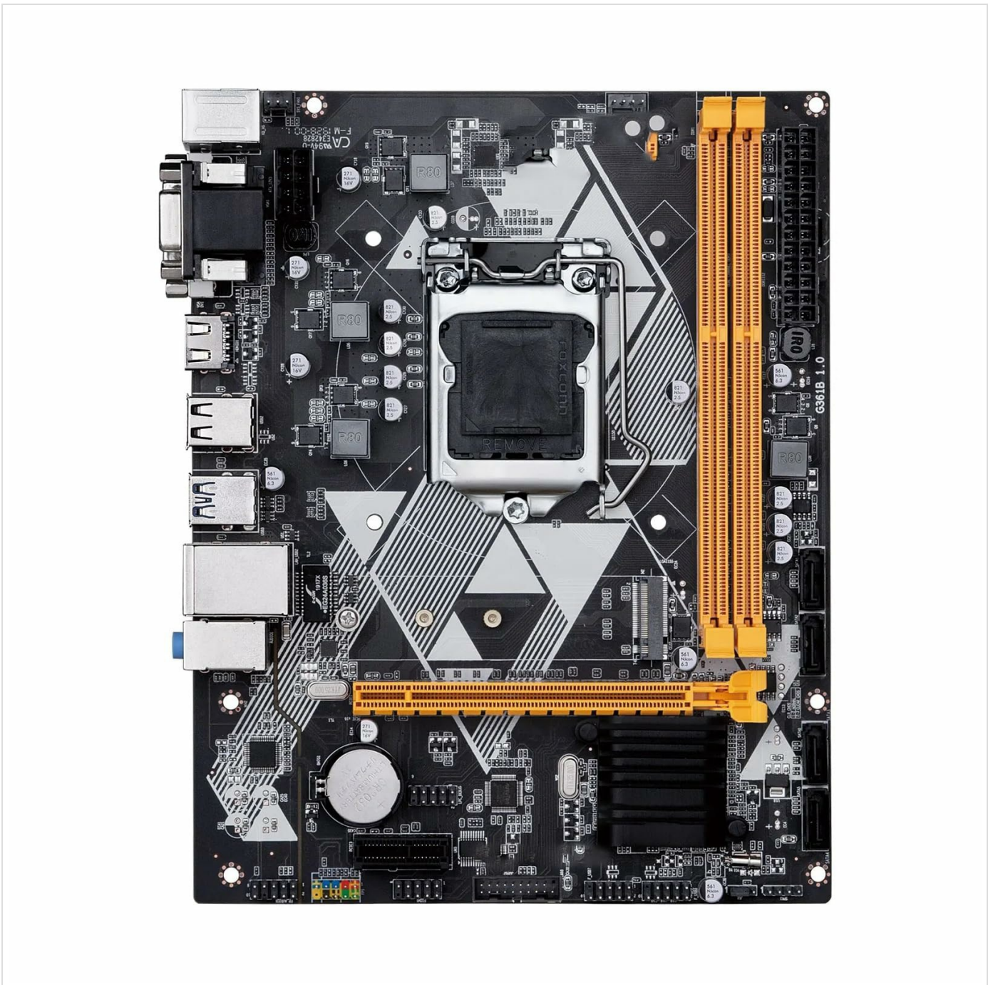
Figure 1: Top-down view of the Generic B85 M-ATX Motherboard. This image shows the CPU socket (LGA1150), DDR3 memory slots, PCI Express slots, SATA ports, and various headers for power and peripherals.
