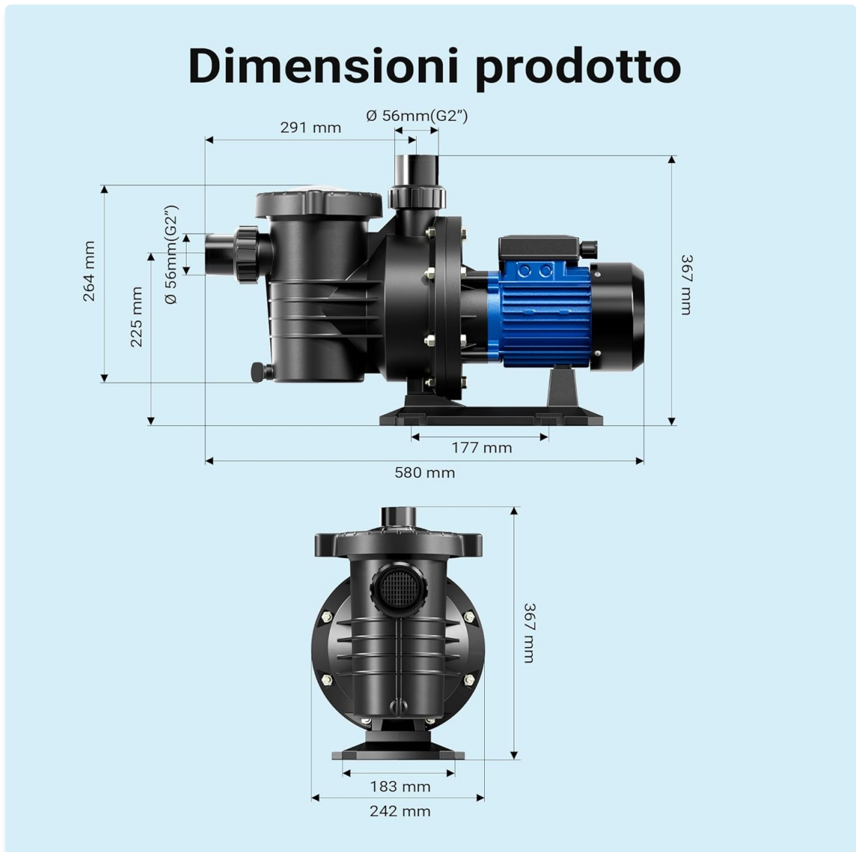
Figure 2: Product Dimensions. This diagram illustrates the pump's overall length (580 mm), width (242 mm), and height (367 mm), along with specific measurements for connections and components.
