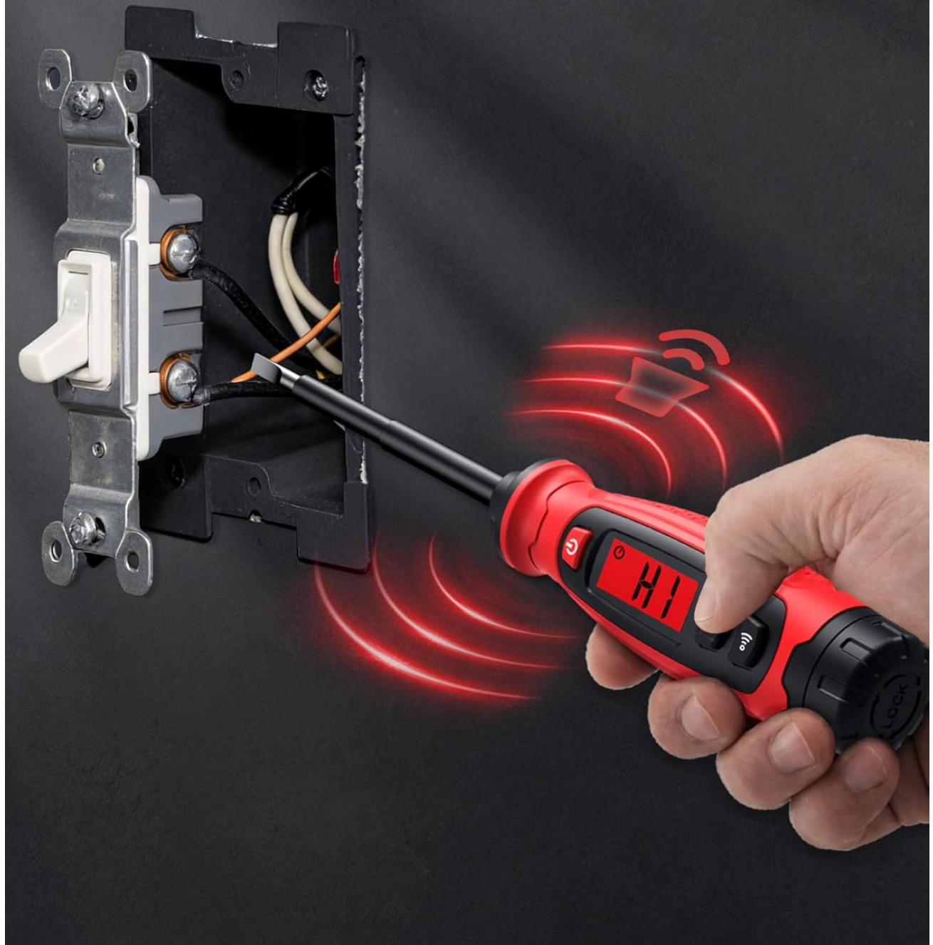
Image 5.2: Non-contact voltage detection near a wall switch.
