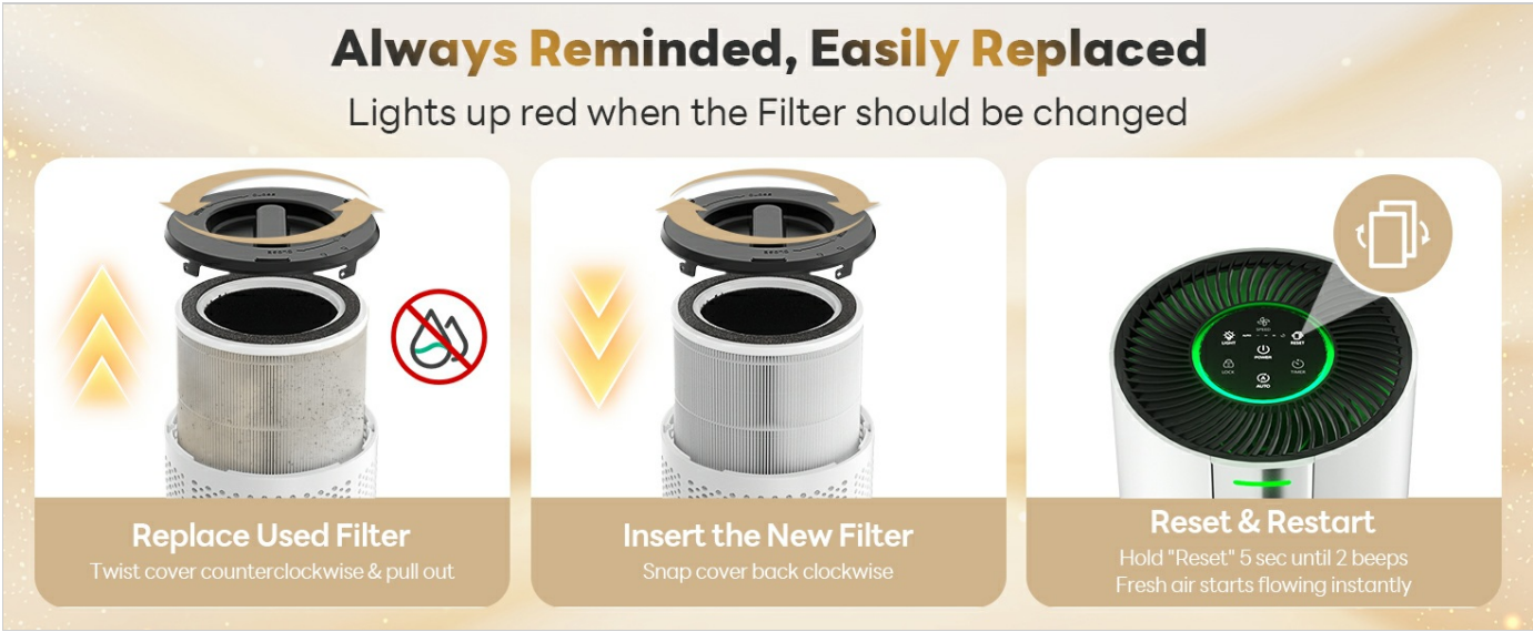
Image: A three-step visual guide demonstrating how to replace the filter: 1) Remove the used filter by twisting the cover counter-clockwise, 2) Insert the new filter, and 3) Reset the filter reminder by holding the reset button.
