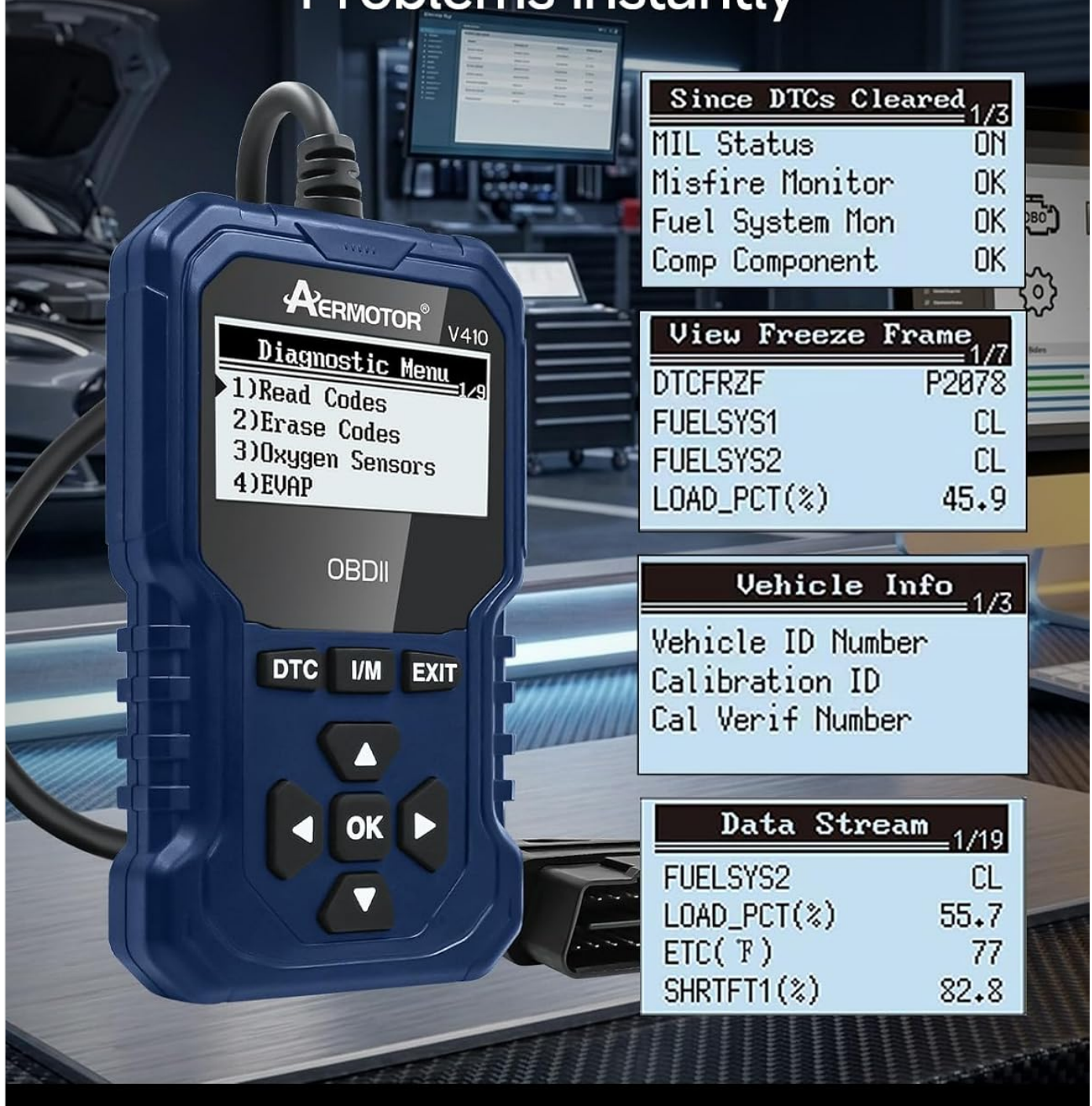
Image: The V410 screen showing real-time live data, including MIL status, misfire monitor, fuel system monitor, and component status, along with vehicle info and data stream values.
