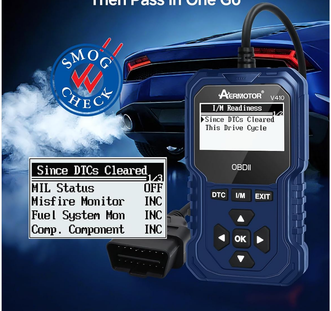
Image: The V410 displaying the I/M Readiness status, indicating whether various monitors are complete or incomplete for emissions testing.
