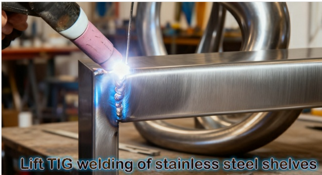
Image: A close-up of Lift TIG welding being performed on stainless steel, showcasing the precision of this welding method.
