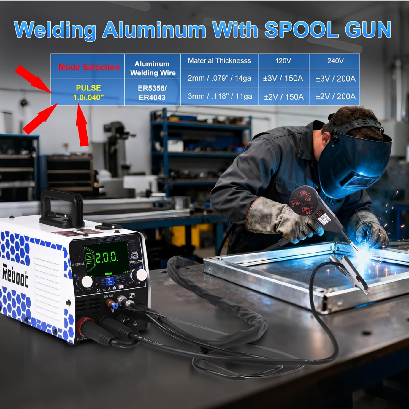
Image: A welder using the RBM2000 with a spool gun to weld aluminum, with a display showing recommended settings for different aluminum thicknesses and voltages.
