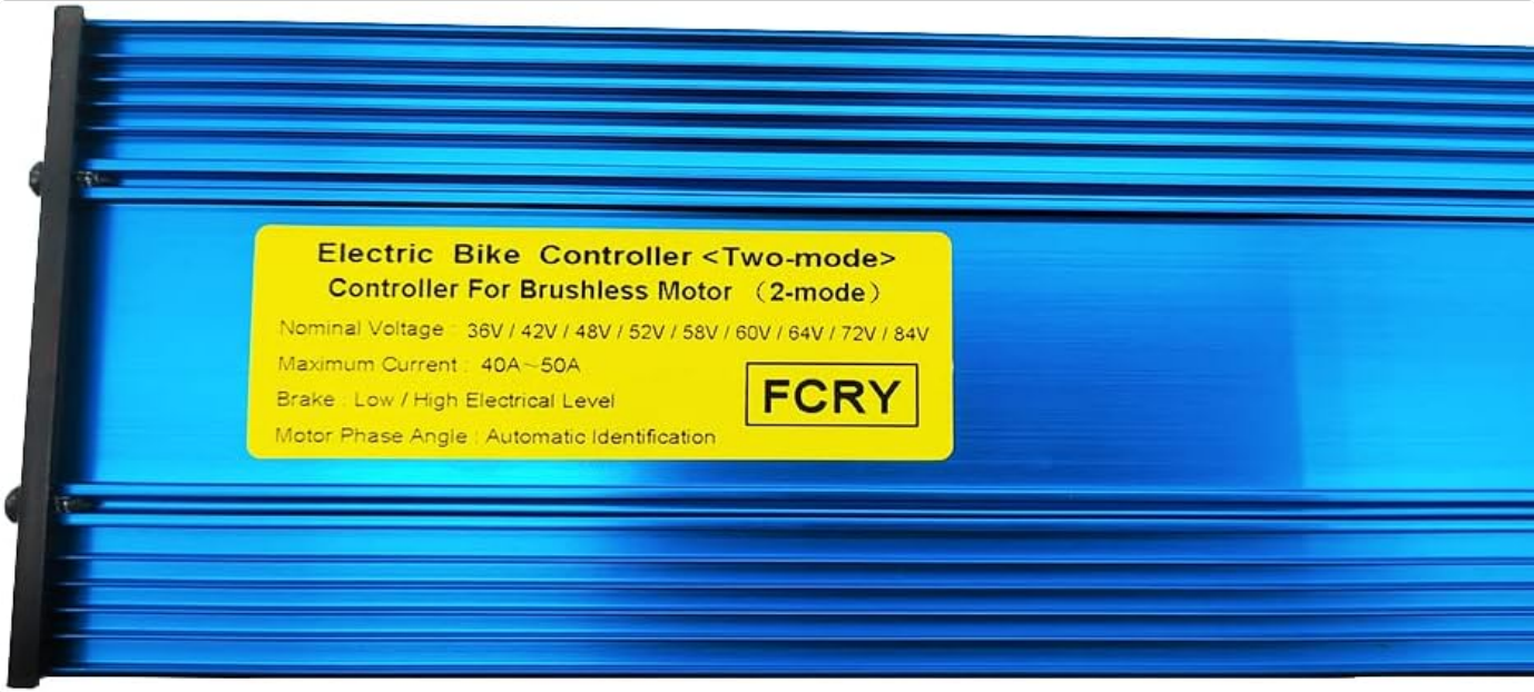
Figure 2: Controller label displaying nominal voltage, maximum current, and brake type.
