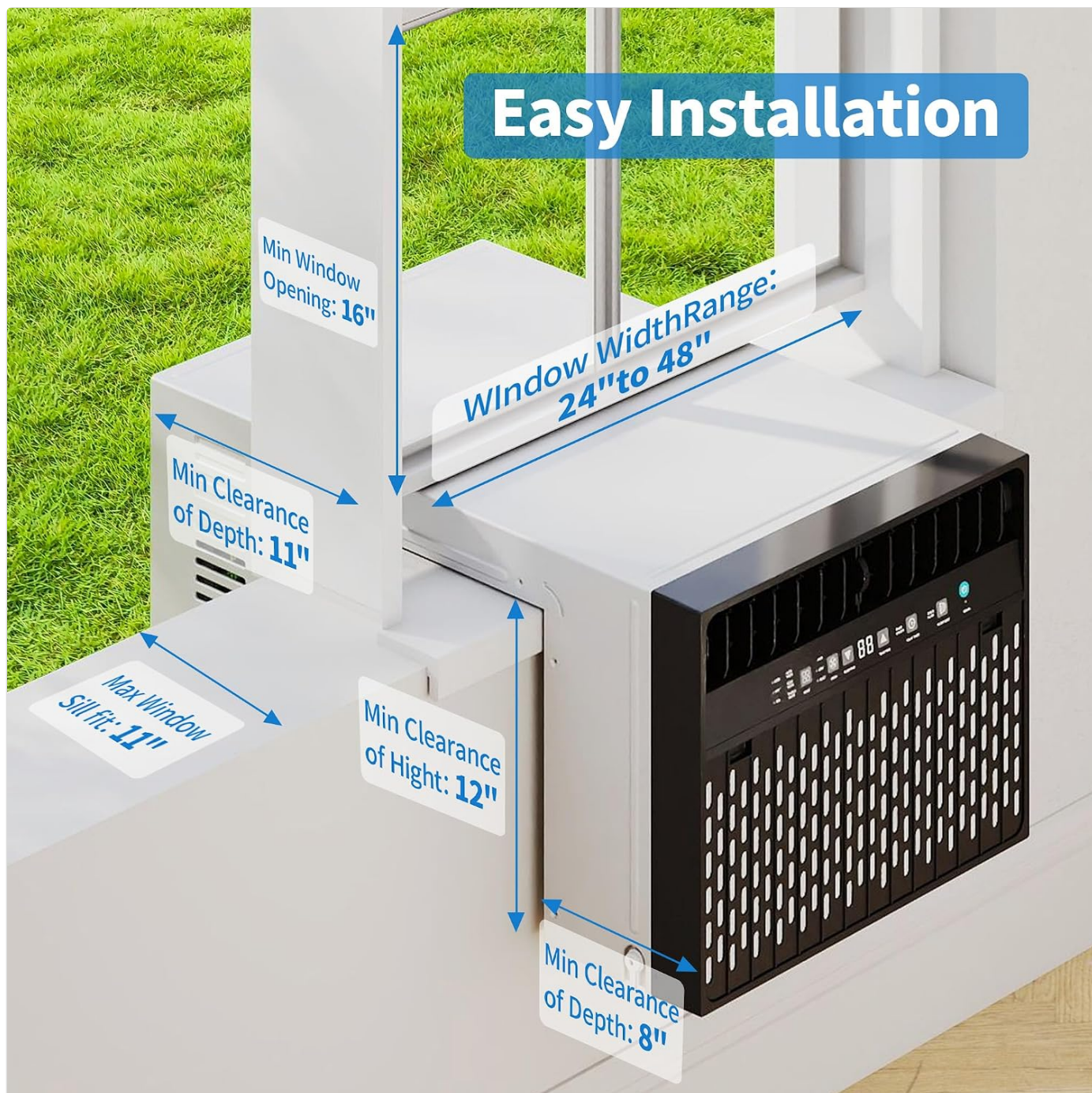
Image: Detailed diagram illustrating the minimum and maximum window dimensions and clearances required for proper installation of the U-shaped AC unit.
