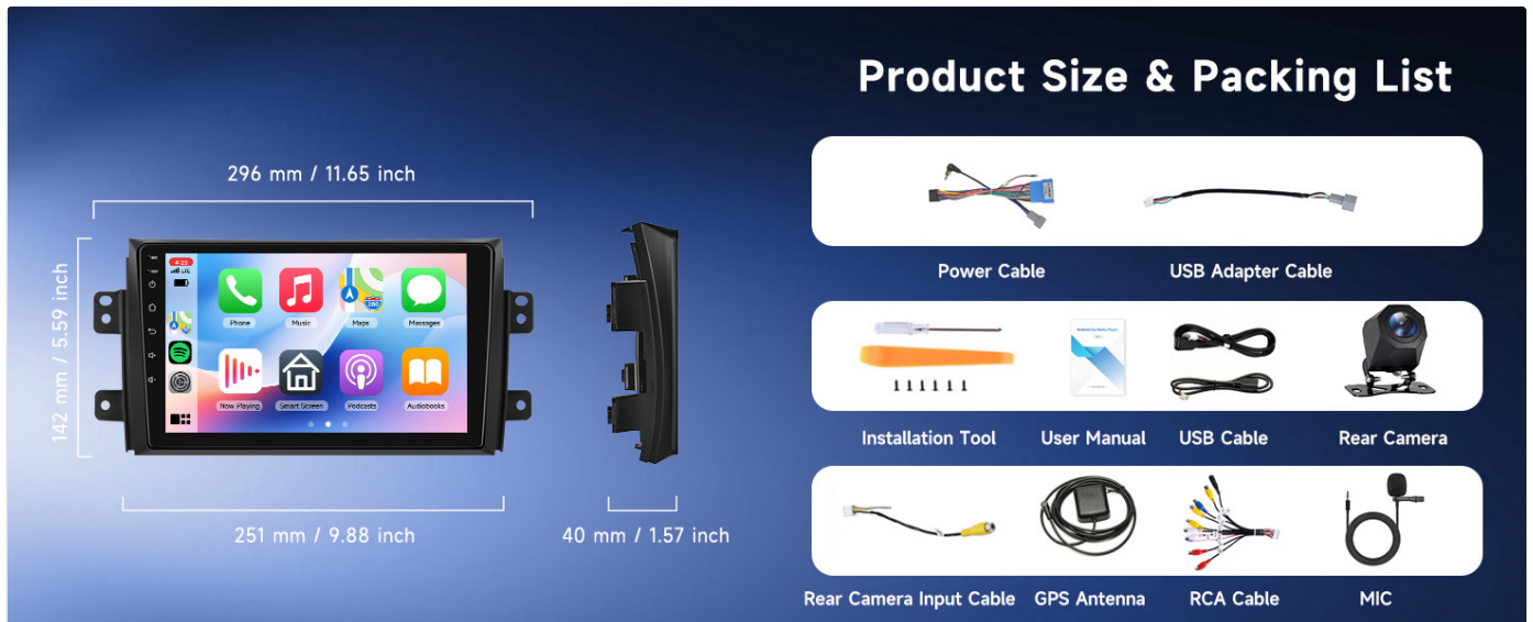
Image: Diagram illustrating the dimensions of the car radio and a visual representation of all included accessories in the packing list.
