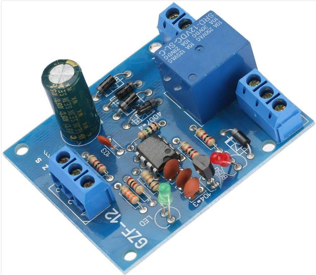
Image: Close-up view of the FTVOGUE Level Controller Switch Module, highlighting the screw terminal blocks for electrical connections.
