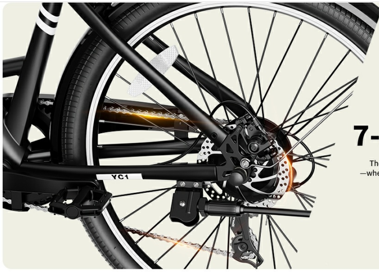
Figure 6: A close-up image of the Jasion Electric Bike's 7-speed drivetrain, including the rear derailleur and cassette. This system allows riders to find their ideal pedaling rhythm for various inclines and cruising speeds.
