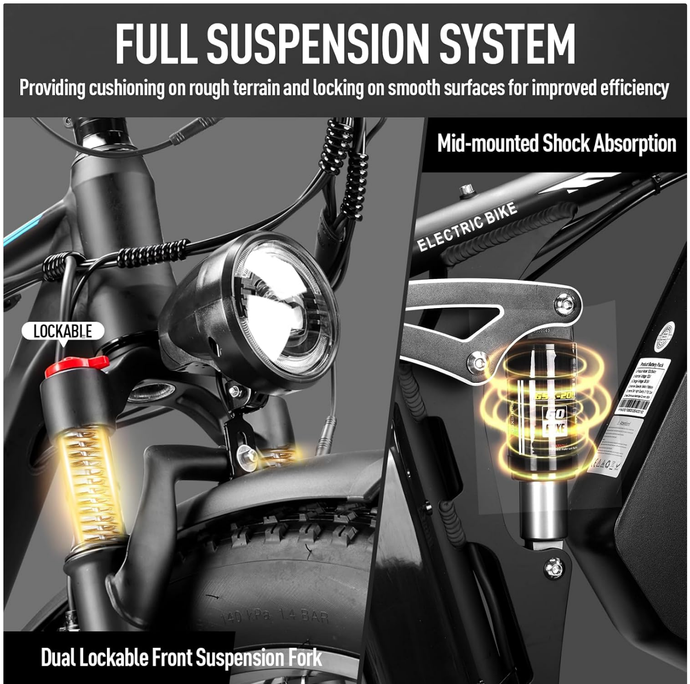
Image: Close-up view of the full suspension system, highlighting the lockable front fork and mid-mounted rear shock absorber.
