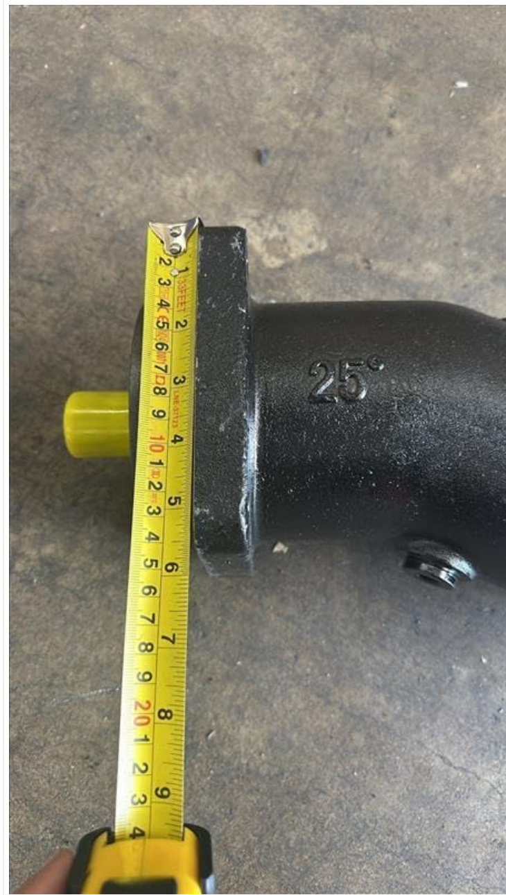
Figure 7.1: The motor with a measuring tape indicating its approximate length. The measurement shows the motor is approximately 15 inches long.
