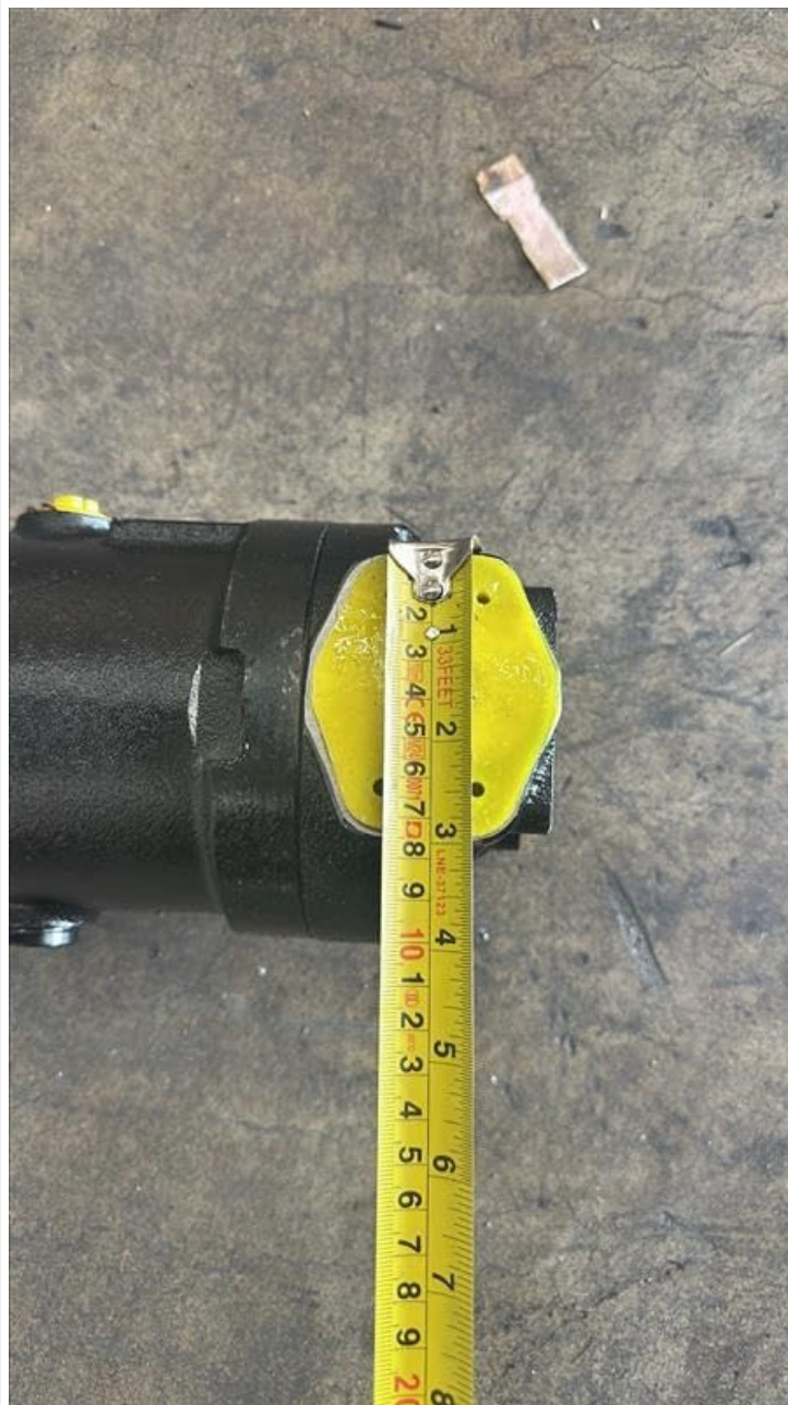
Figure 7.2: The motor with a measuring tape indicating its approximate diameter/width. The measurement shows the motor is approximately 5.5 inches wide.
