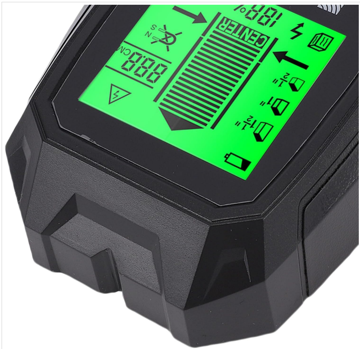
Figure 4: Close-up of the LCD display showing a detected object with center indication and signal strength.
