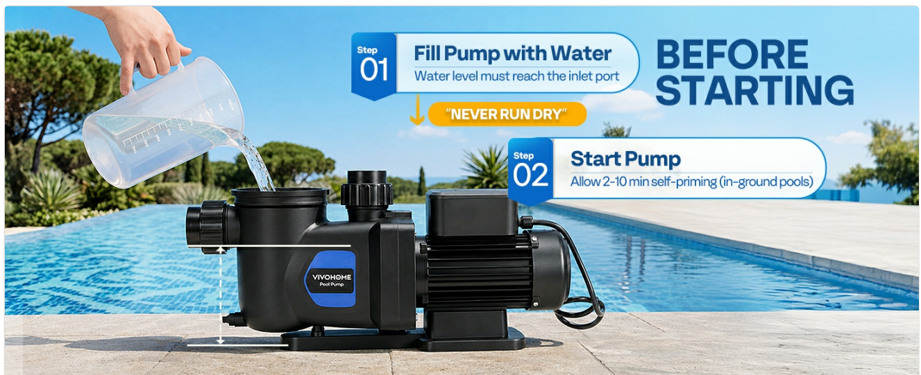
Figure 4: Before Starting. This image visually guides the user to first fill the pump with water up to the inlet port and then start the pump, allowing 2-10 minutes for self-priming.
