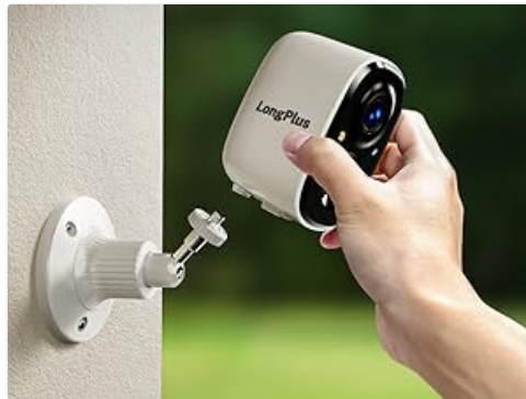
Image 3.3: Demonstrating how to attach the camera to its wall mount.
