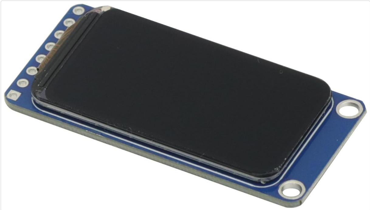
Image: Front view of the 1.47 Inch TFT IPS Display Module, showing the display area.
