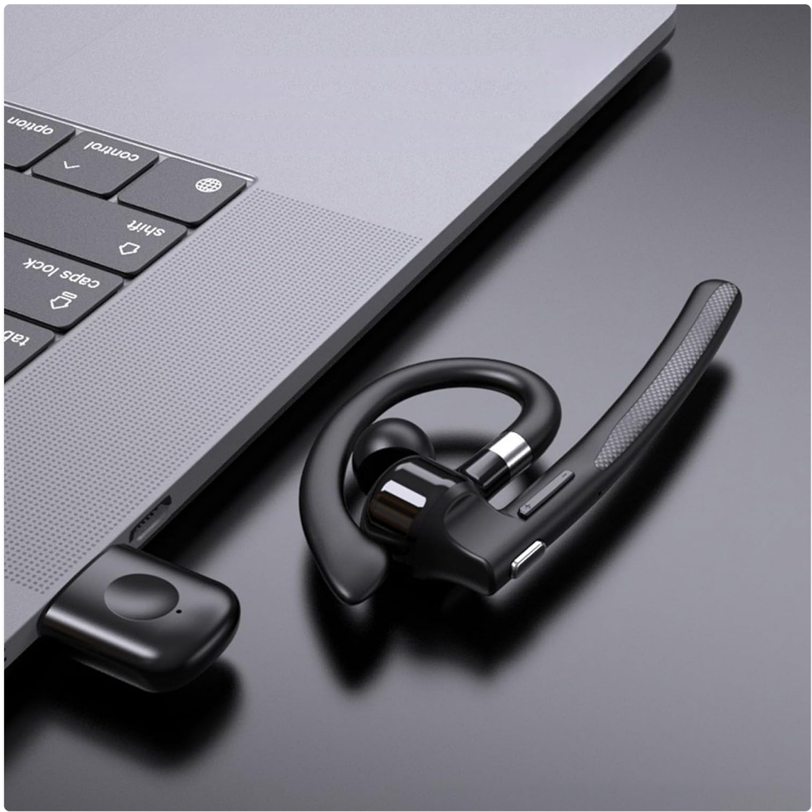
Image: Illustration of the headset's rotatable earpiece and ear hook for left or right ear wearing.
