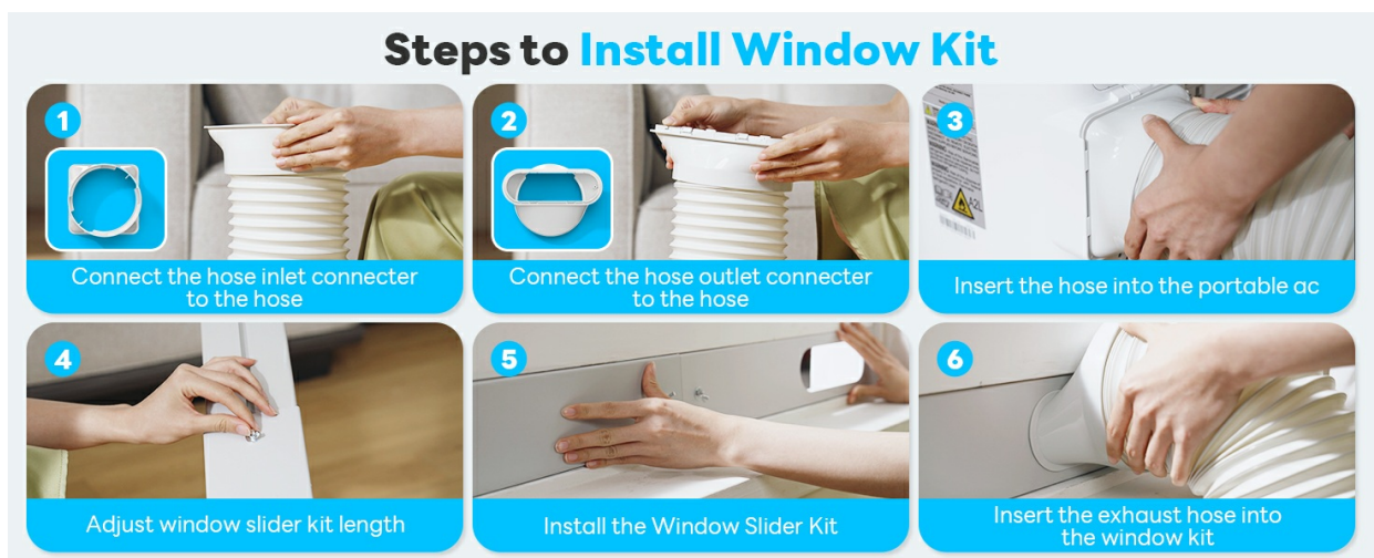
Figure 2: Visual guide for installing the window kit and exhaust hose.
