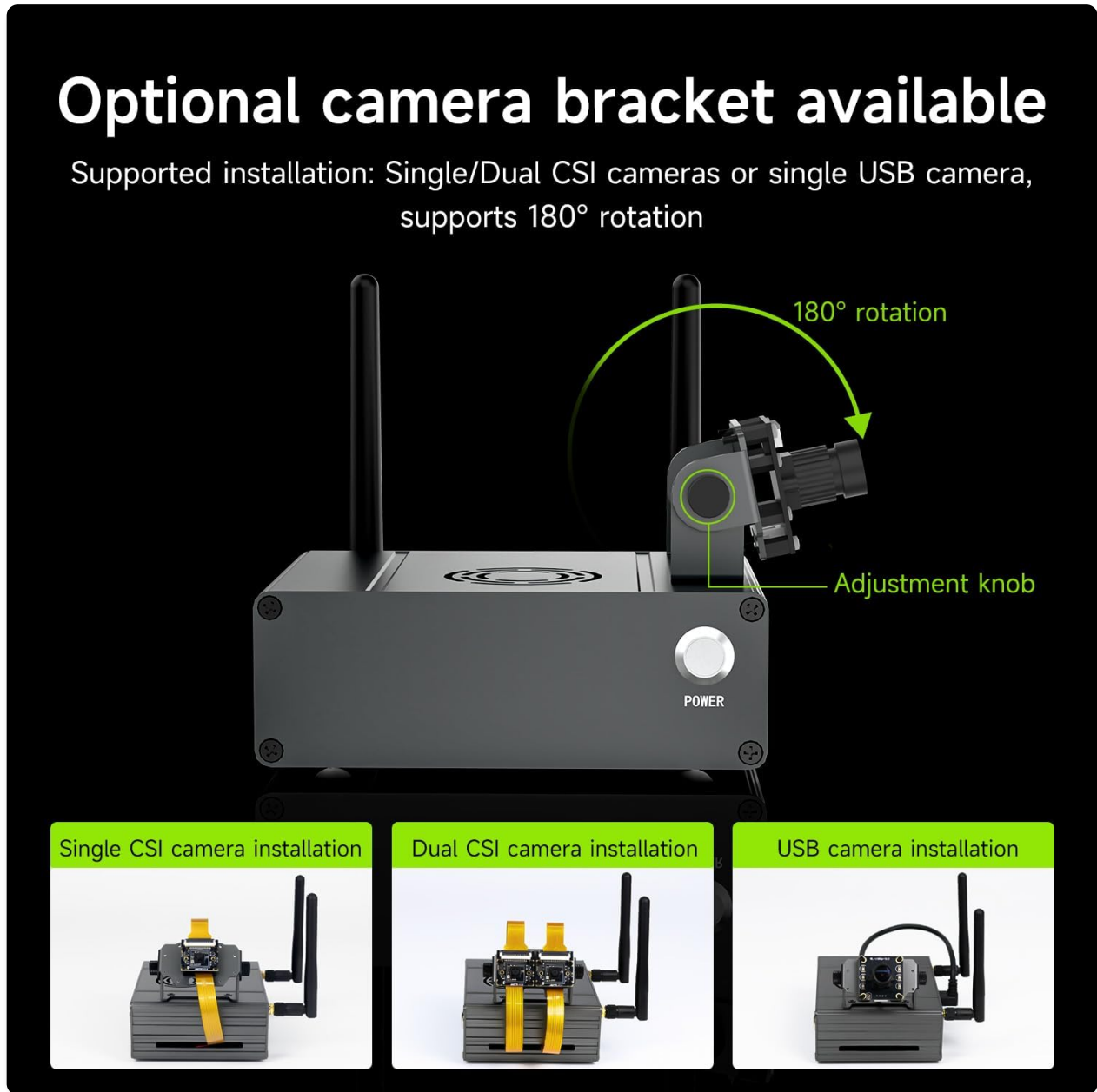
Image: The camera bracket with an adjustment knob, illustrating its 180° rotation capability for flexible camera positioning.
