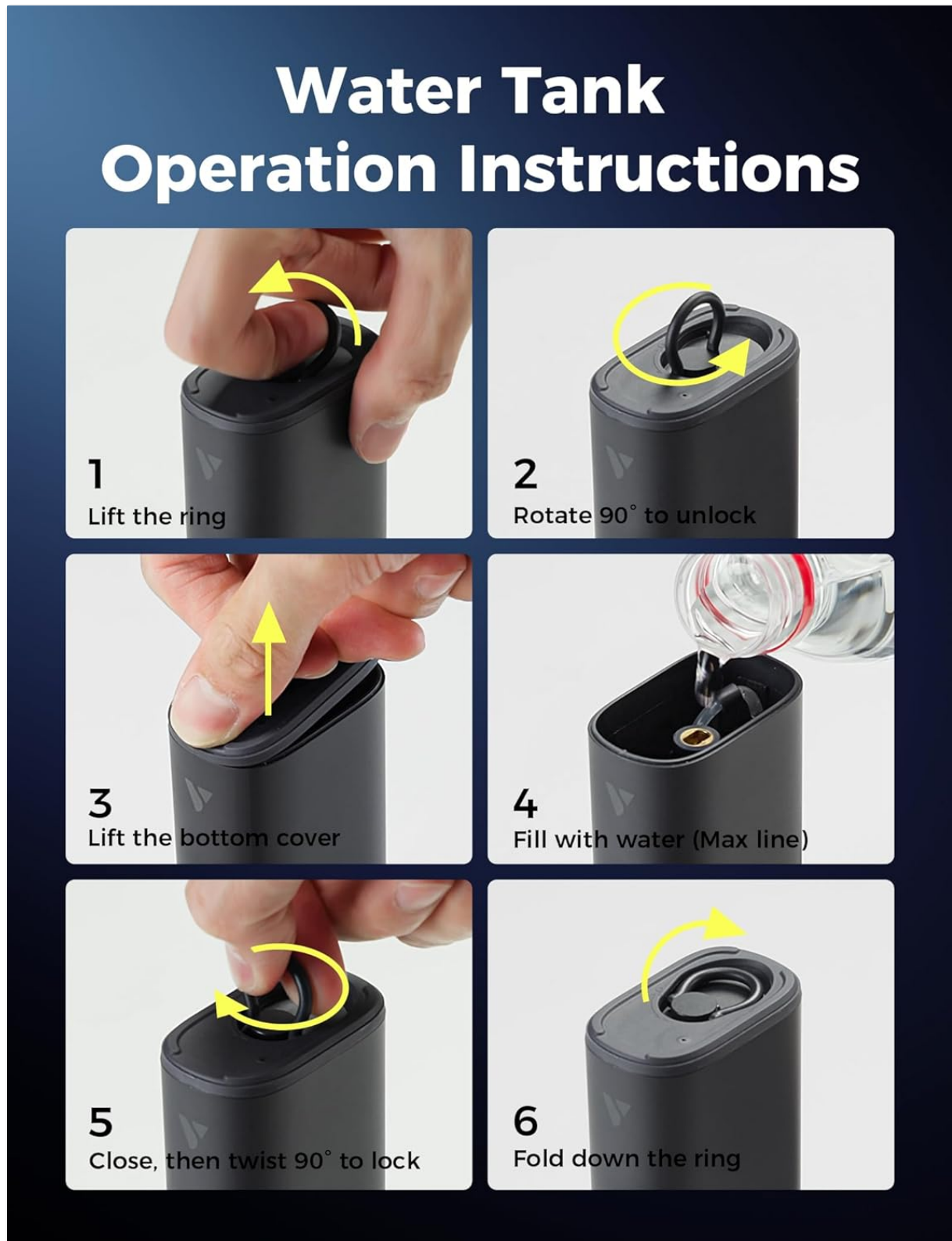
Image 5.2: Water Tank Operation Instructions.
