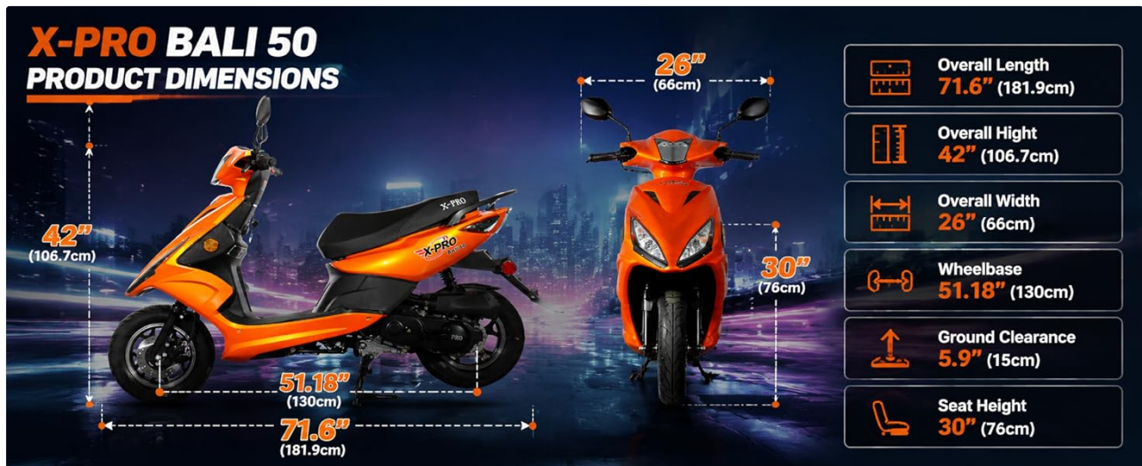
Figure 7.1: Detailed product dimensions of the X-PRO Bali 50cc Moped.
