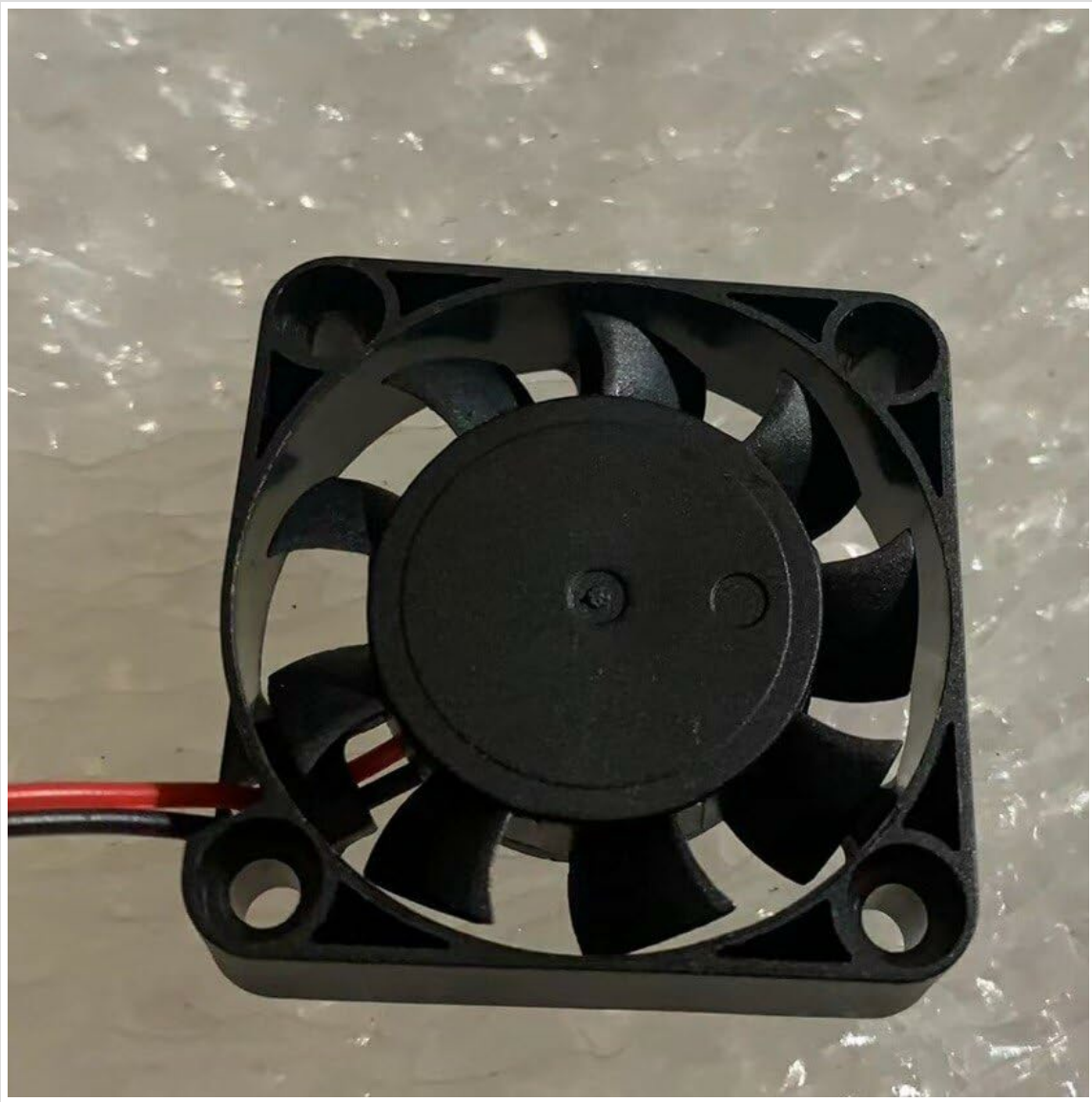
Image 2: Close-up view of the Shrandi RDH4010B fan, highlighting the red and black power wires extending from the fan frame. This image helps in identifying the wiring for installation.
