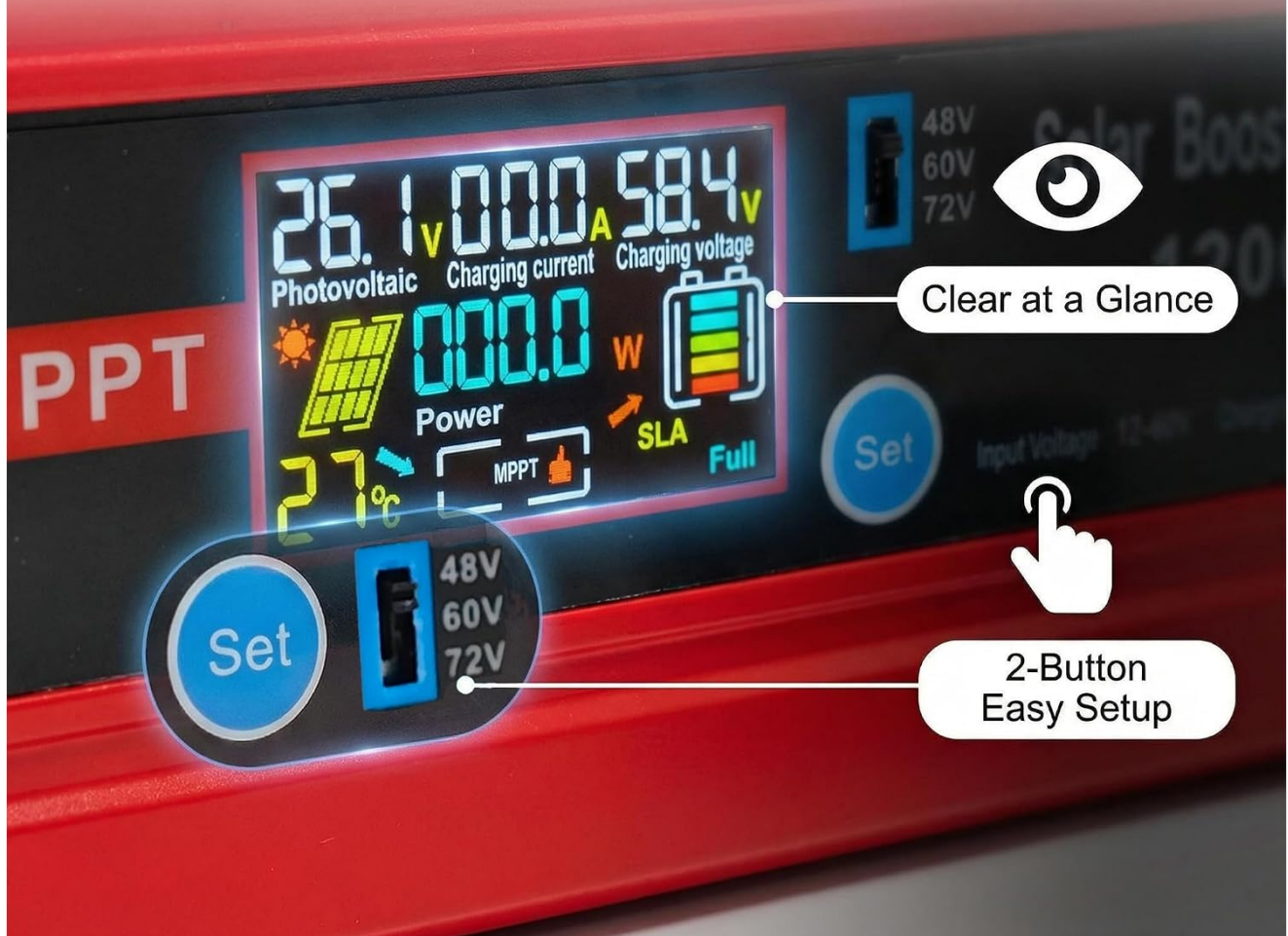
Figure 2.2: Detailed view of the controller's HD LCD color screen, displaying photovoltaic voltage, charging current, charging voltage, power, and battery state. The 'Set' button and voltage adjustment switch are also visible.
