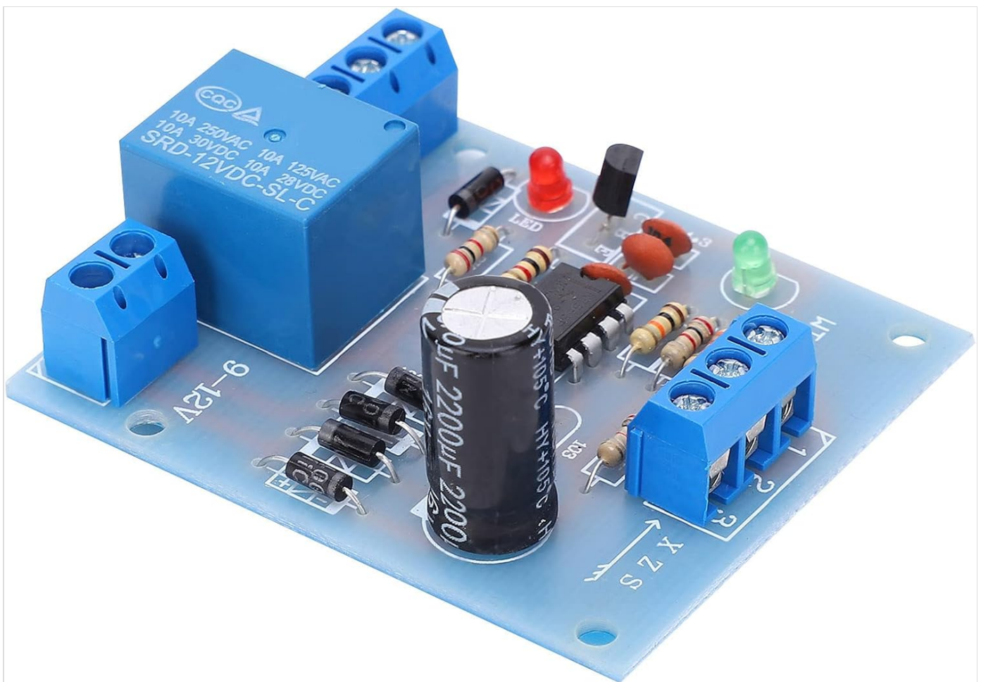
Figure 6.1: Angled view of the FTVOGUE 12V Liquid Water Level Controller Module, highlighting the electronic components and relay.
