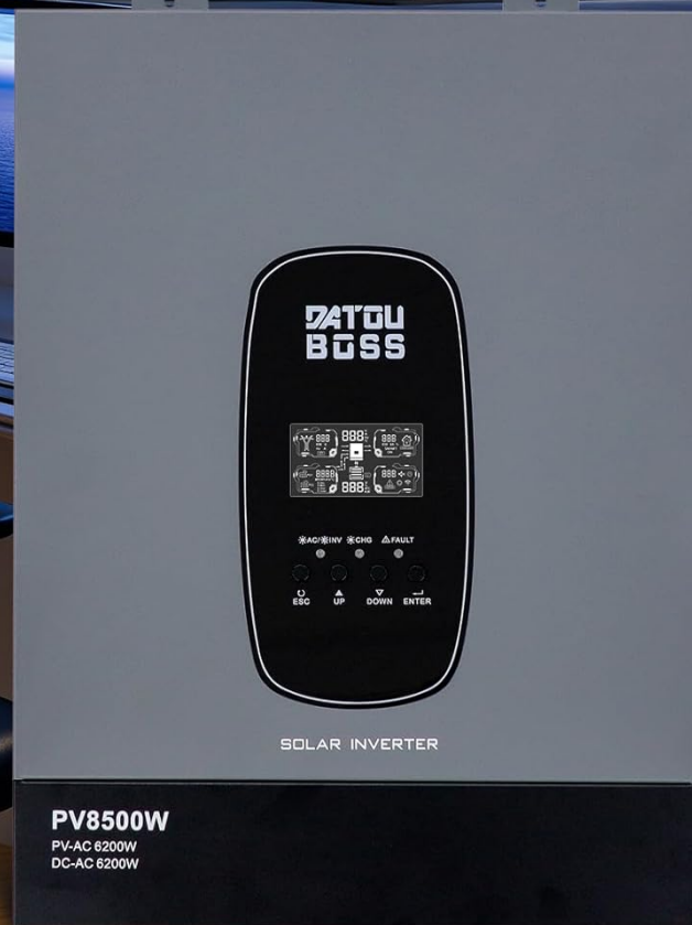
Figure 1: DATOUBOSS 48V 6200W Hybrid Solar Inverter. Key specifications include 6200W rated output, 8500W max PV input, 48V 120A DC input, 27A max PV input current, 230VAC 50/60Hz AC output, 500V max solar voltage, -10°C to 50°C operating temperature, 100A/120A DC max charging/discharging current, and IP54 ingress protection.
