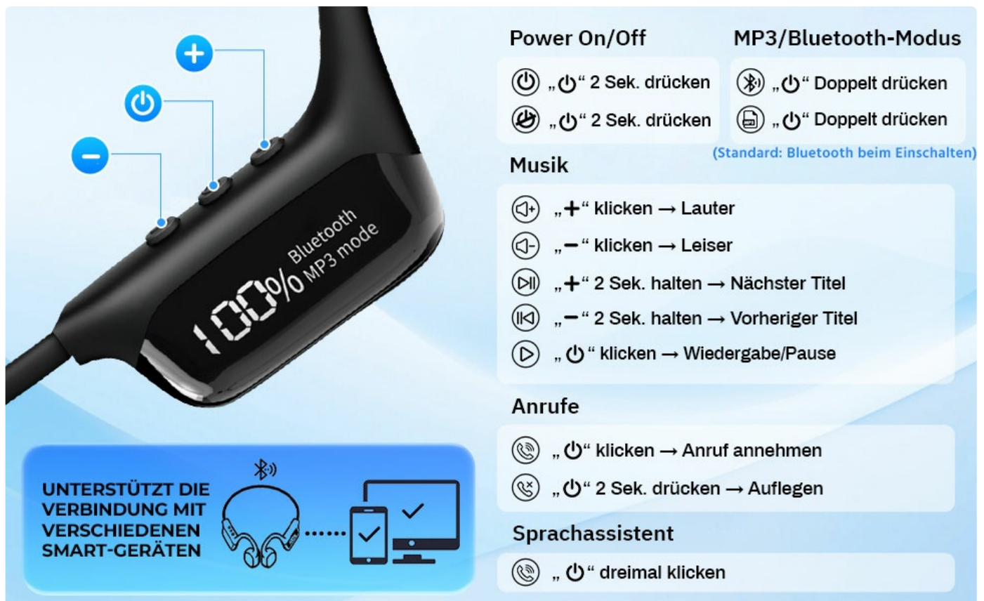
Image 3.1: Detailed diagram of the control buttons and their functions for the Aiandcc S10 headphones.
