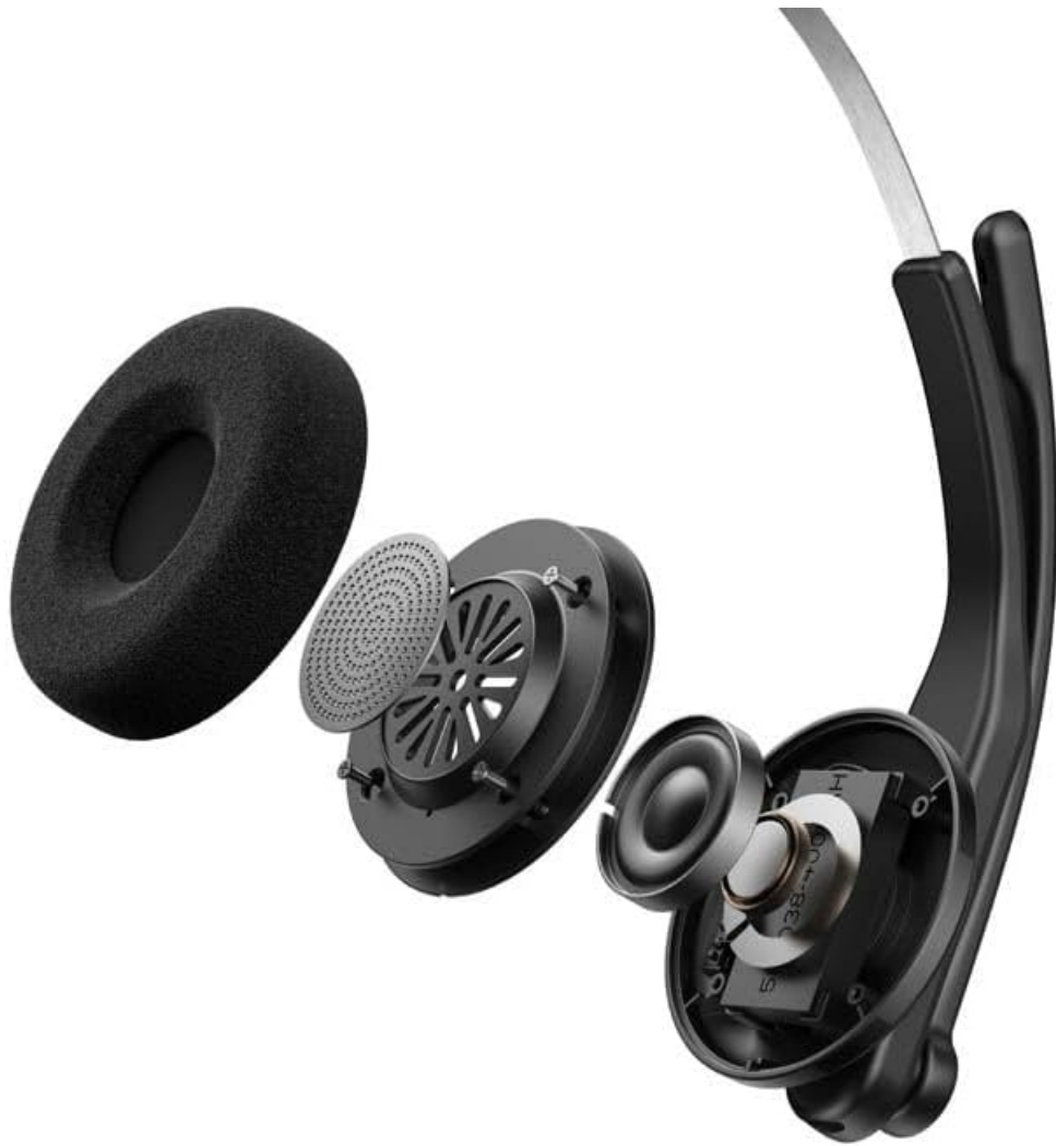
Figure 3.4: Exploded view showing the internal components of the earcup, including the 30mm dynamic driver.
