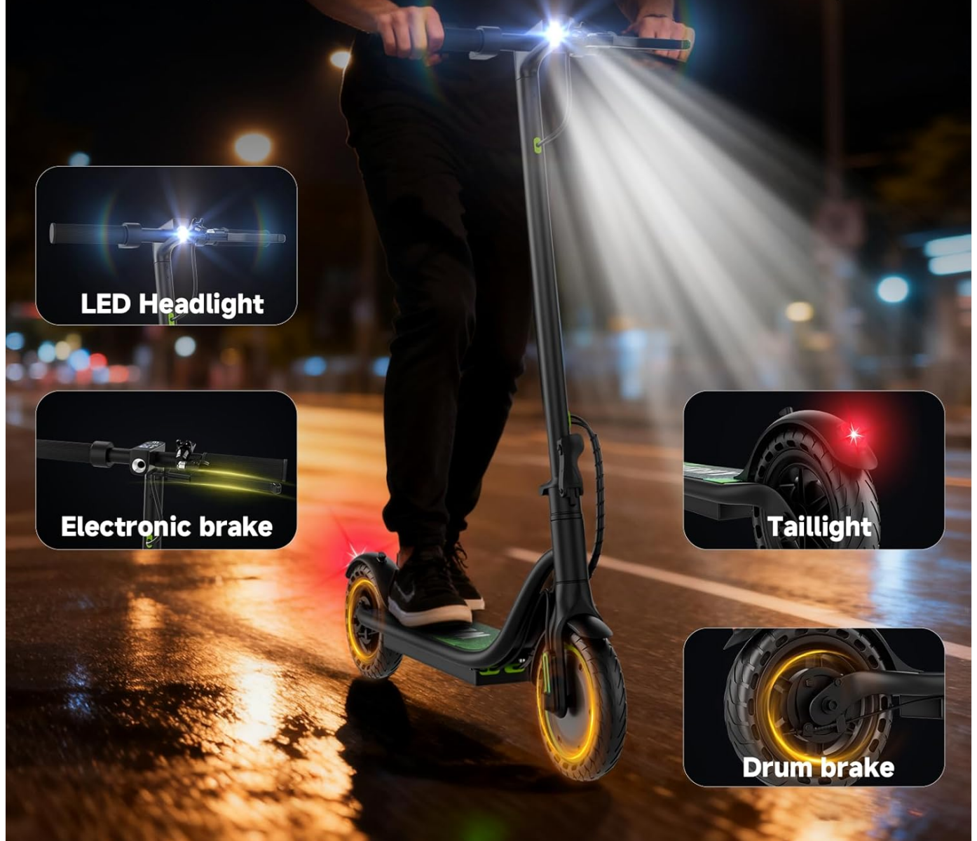
Figure 2.4: Dual braking and lighting system for enhanced safety.
