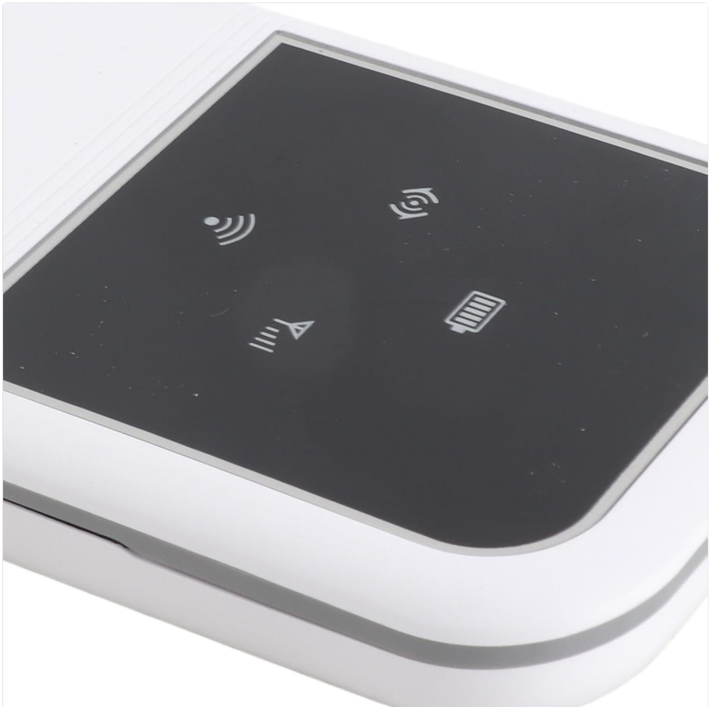
Image: A close-up view of the POENVFPO 4G LTE H80 Wi-Fi Hotspot's black display panel, featuring illuminated icons for Wi-Fi signal strength, network connection status, and battery charge level.
