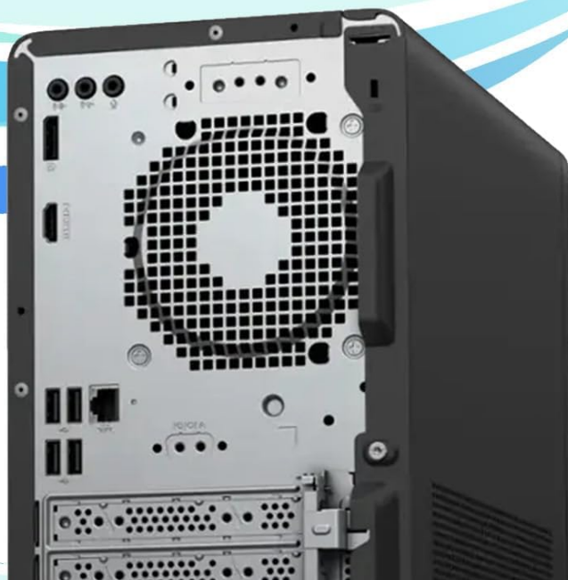
Image 2.1: Front and rear ports of the HP OmniDesk M02 Business Tower Desktop. This image illustrates the various connectivity options, including USB Type-C, USB Type-A, HDMI, DisplayPort, and RJ-45 Ethernet ports, facilitating easy connection of peripherals and network devices.
