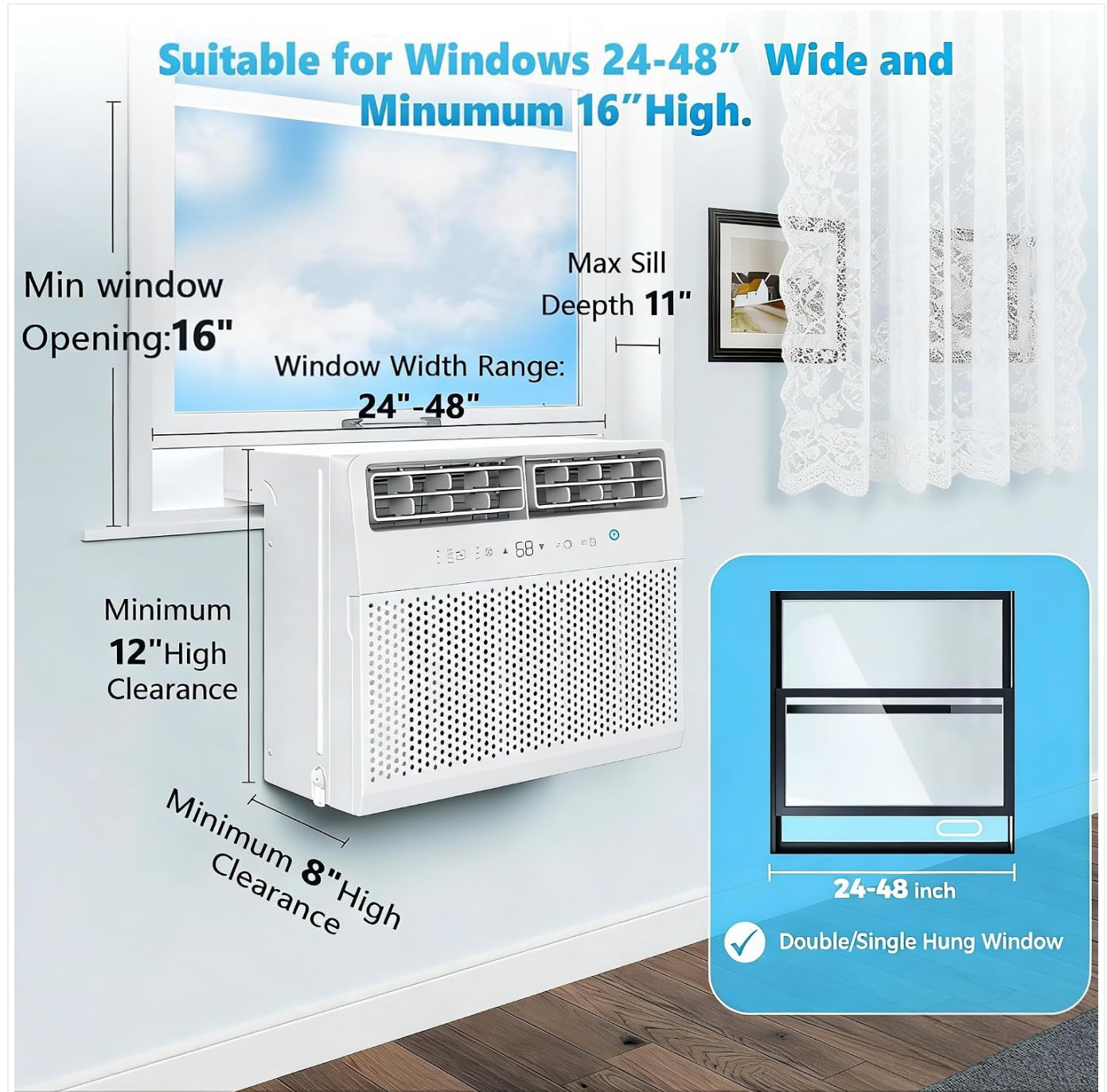
Figure 4.1: Window dimension requirements for installation.
