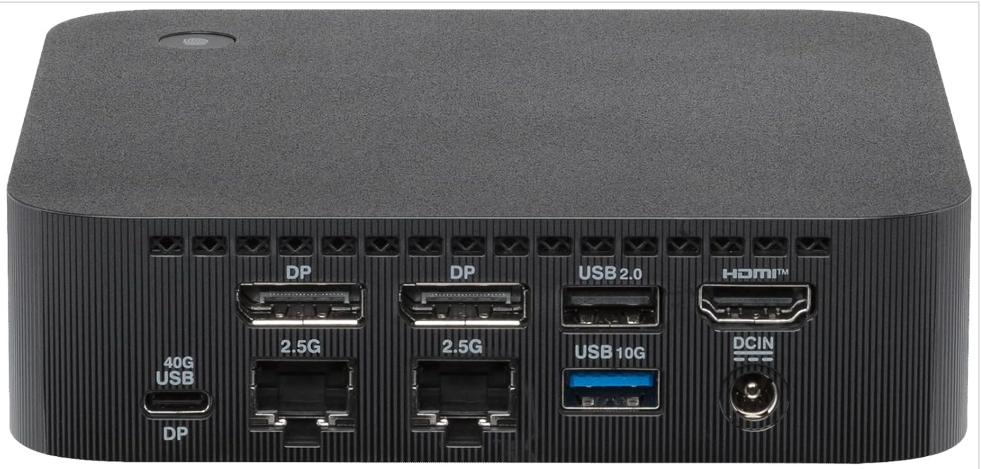
Image: Rear panel of the Mini PC, featuring DisplayPort, 2.5G LAN, USB 2.0, USB 10G, HDMI, DC-in, and a 40G USB-C port with DisplayPort functionality.
