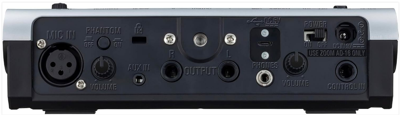
Image 3.2: Rear view of the Zoom V3 Vocal Processor, showing all input and output ports.
