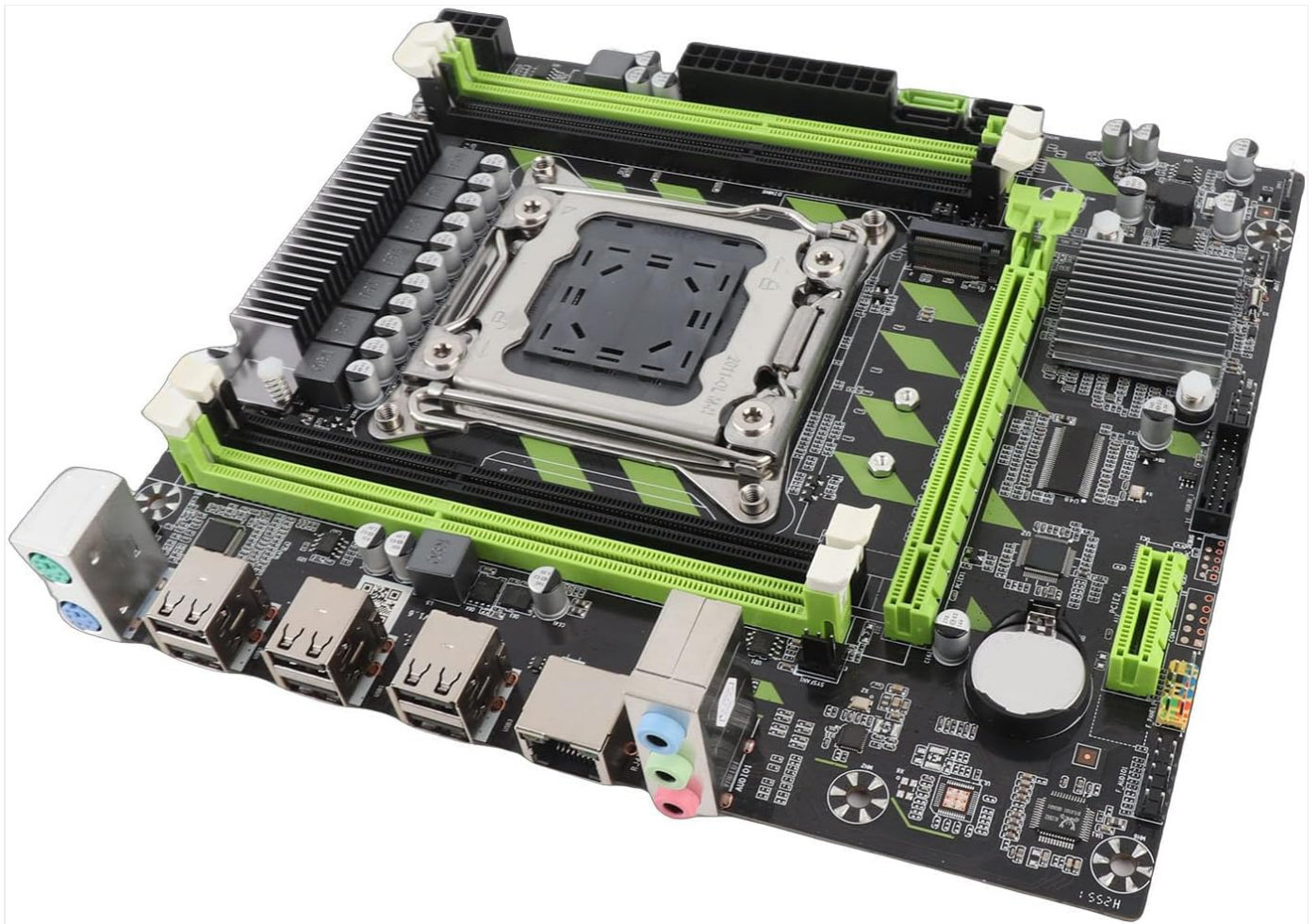
Image 3.1: Rear I/O Panel. This image displays the input/output ports located at the back of the motherboard, including multiple USB ports, a Gigabit Ethernet port, audio jacks, and legacy PS/2 ports for keyboard and mouse.
