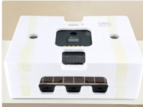
Styrofoam cover for additional insulation.
