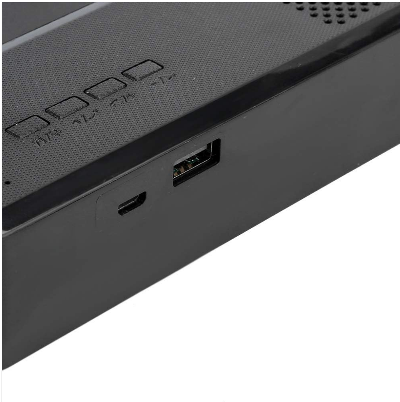
Figure 2: Control panel and ports. This image shows the USB port, charging port, and control buttons for power, volume, and playback functions located on the speaker unit.
